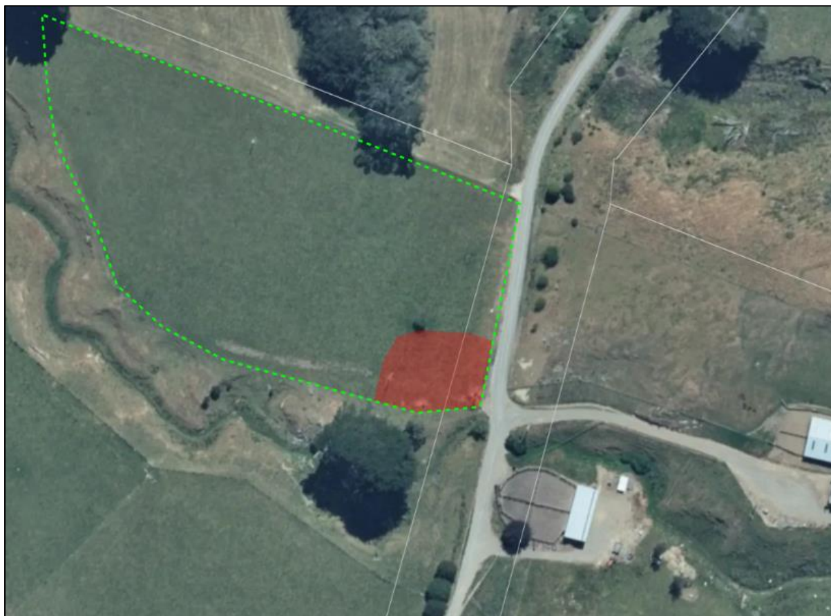
Figure 11: Recommended buffer area (shaded in red) where excavations should be avoided.
