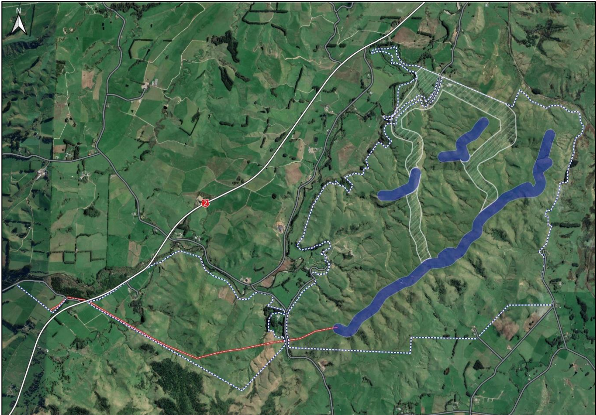
Figure 2: Project overview showcasing the Turbine Envelope Zone (blue shaded area), Turbine Exclusion Zone (white hashed area), and Transmission Corridor (red dashed line). All turbines and infrastructure will be located within these areas.
